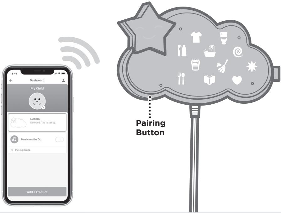
Open the Fisher-Price® Smart Connect™ app on your device (not included) and touch the Lumalou™ icon on the Smart Connect™ dashboard. Be sure your device is within approximately 1,8 meters - 6 feet of the Lumalou™ unit to pair.
