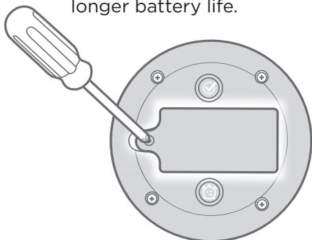
Loosen the screw in the battery compartment door and remove the door.
