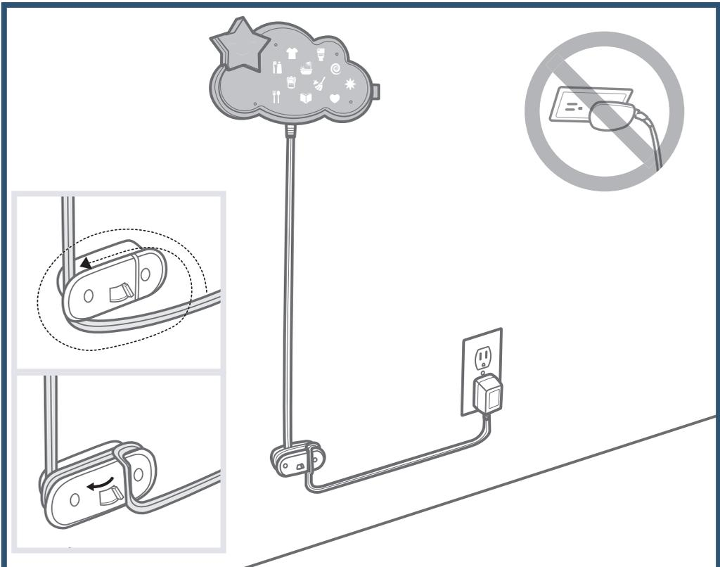
**IMPORTANT!** Make sure the cord is taught between the Lumalou™ unit and cord wrap cleat. Excess cord can form loops and present a strangulation hazard.
